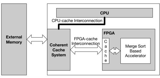
Target CPU-FPGA heterogeneous architecture
