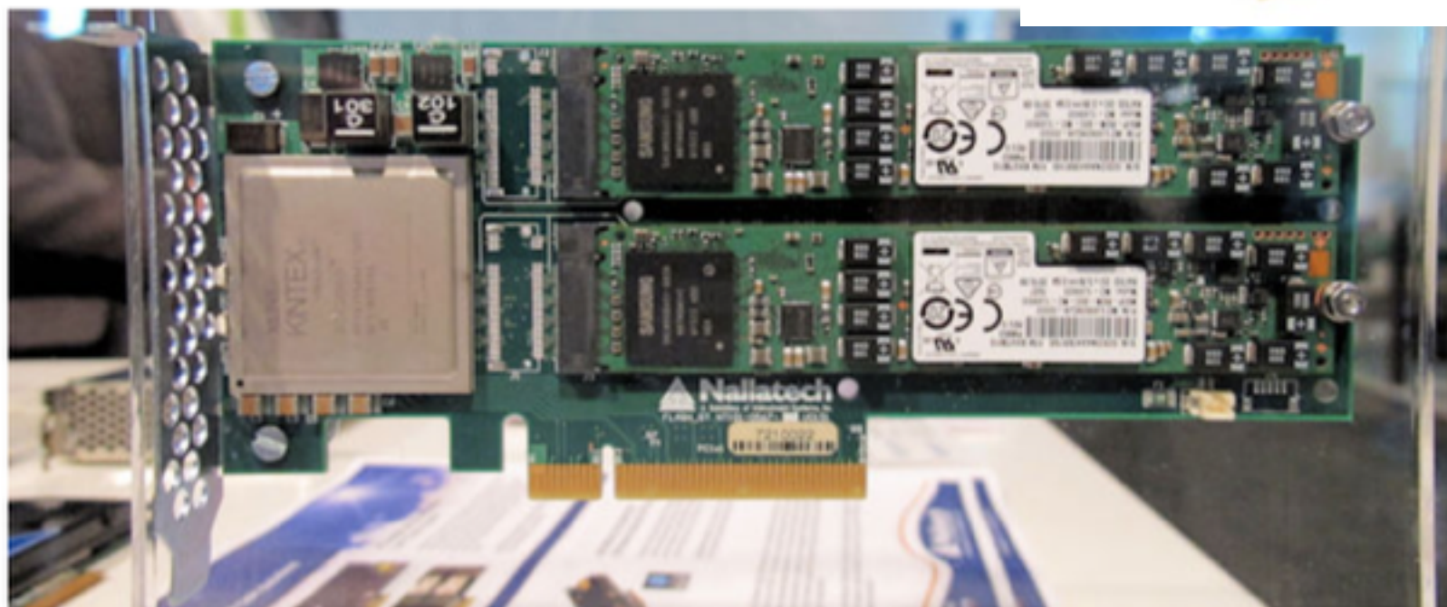
Nallatech CAPI Flash Accelerator based on a Xilinx Kintex UltraScale KU060 FPGA
